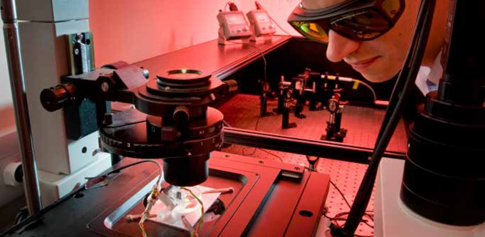
Using lasers to levitate and manoeuvre cloud droplets, in order to investigate their surface chemistry
